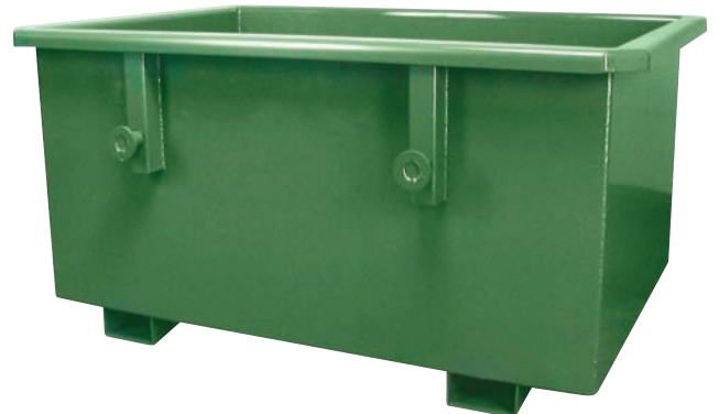
Extra heavy duty container fabricated from 3/8" plate. Designed for transport with overhead crane and to be emptied with rolover attachment on forklift. Used by bearing manufacturer.
